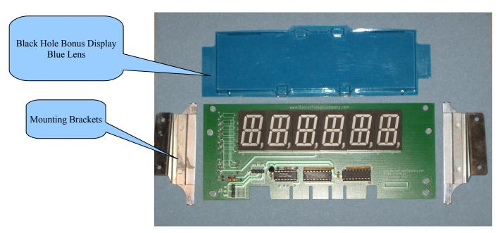
Slide the mounting brackets on the edge of the Display and over the lip of the lens. (You can use a piece of Scotch tape to hold the lens to the Display before installing the brackets)
